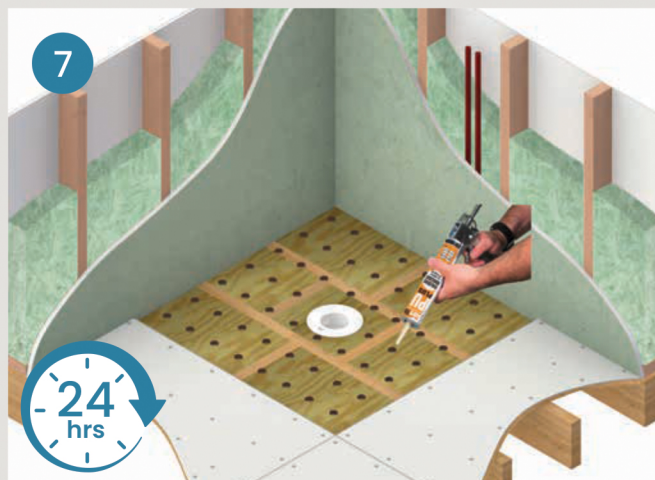
7 Fix Tile & Slate to floor outside shower pan area. Apply adhesive - 24 hour cure time.
