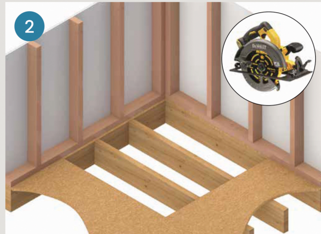
2 Cut out 20mm flooring and remove.
